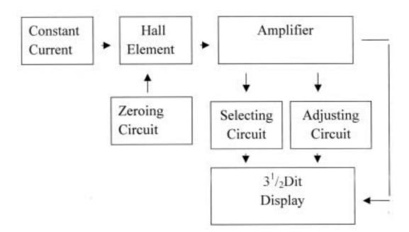
When Hall element H is placed in the magnetic induction field with intensity B and connect a constant current I through end 1 and 3,then a voltage VH would be occurred between end 2 and 4, after amplified by the arithmetic amplifier, it outputs to the display and the relevant readings of magnetic field intensity will be displayed on the LED.
