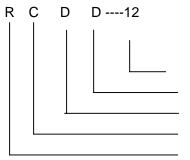
Adaptive belt width Electric series & air cooling, auto removing Electro-magnetic Magnetic separator For mine
