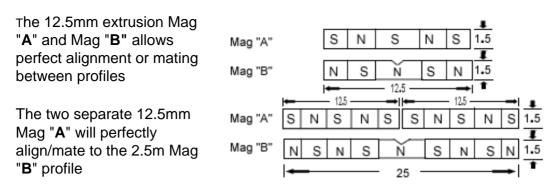
The magnet to magnet applications are most useful for fixing of posters and graphics in display systems. In addition to Mag "A"/Mag"B", other types of self aligning systems can be manufactured on request.
